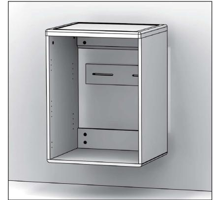
NOTE: For added stability, screw two additional screws into studs through the the top spanner (h) of the cabinet.
